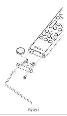
**NOTE:** Use only the tool supplied with the unit to remove the screw to avoid damage to the hex screw.
